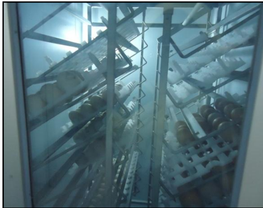
GAMBAR 16.5 Incubator Setter Berkapasiti 2,500 Biji Telur Ayam
