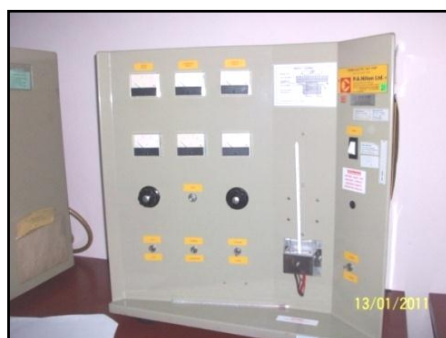
Thermo Electric Heat Pump, Di UiTM Shah Alam
